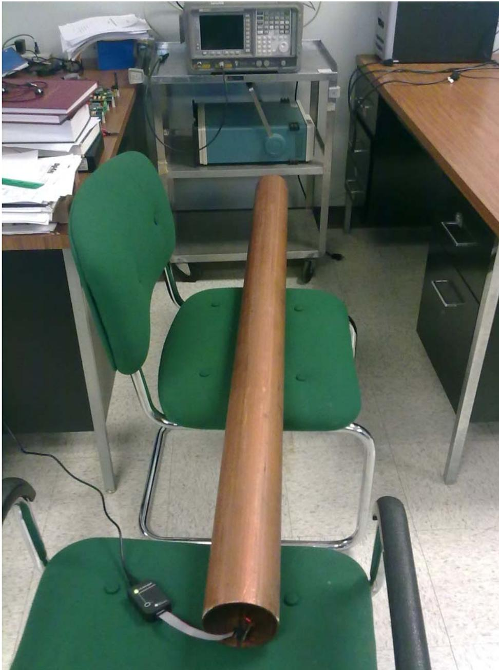
Fig. 25 Probing the electromagnetic wave inside a pipe.
