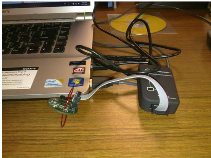
Fig. 23 Programming the transceiver with CC Debugger.
